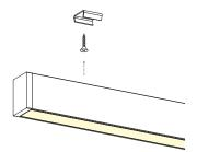
Steel clip for snapping onto flat surfaces. The clip hooks onto the rear slots, which will be perfectly adhered to the surface. 12xM2.5 screws included.
